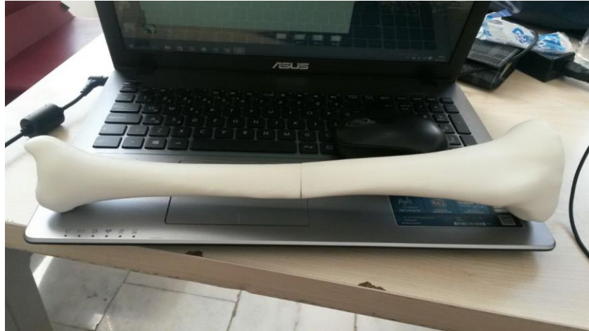
Figure 5. Tibia after printing
